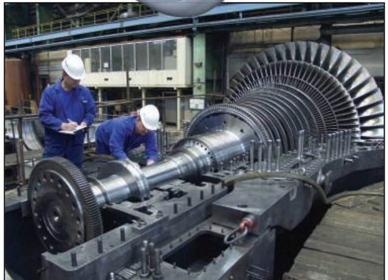
FIGURE 4. The steam turbine driver shown here is a horizontally split machine with many axial-flow stages. Steam turbine drivers offer speed match (direct drive, without gear unit) and variable-speed drive operation
